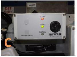
Photo C – Once the alarm has been silenced, the red alarm light will remain lit until the Cube is at less than 85% fill capacity.
