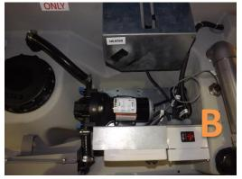
Photo C - The TD10 is equipped with a timer that will automatically shutoff the pump after approximately six minutes of run time, or when a transaction is completed via entry in to the automated fuel management system interface.
