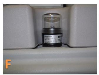
Photo F – To prevent spills, the Cube is constructed with double walls. If a leak within the inner wall were to occur, fluid would be visible in the sight glass. It is recommended that the sight glass be checked on a periodic basis.
