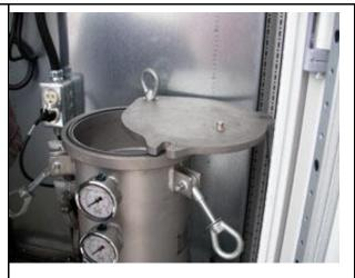
Step 5: Carefully pry filter loose.
