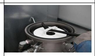
Step 6: Remove the filter from the inlet tube.
