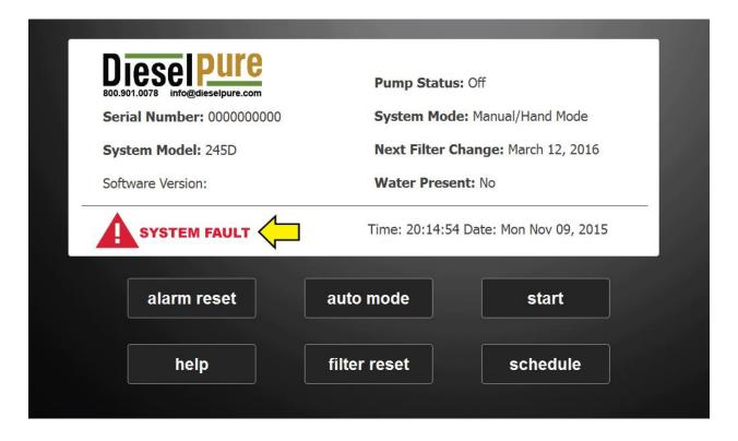
The system fault icon will be shown on the screen when a sensor detects an unsafe or abnormal operating condition. These conditions can include a fluid leak, pump fault, and general system faults.
