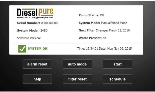
The primary user interface for the DieselPure system is a resistive touch-screen display. This GUI starts automatically when the system is powered on.
