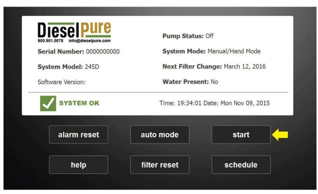
The start / stop button is used to start and stop the pump independant of any schedule cycles.
