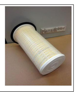
Step 8: Insert the new DieselPure™ Efficiency SAE compliant filter
