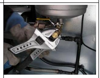
Step 4: Drain off water from fuel through the oily water filter and into a waste container.
