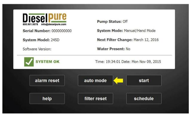
The auto mode button is used to switch between auto mode (scheduled run cycles) and manual (hand operated mode).
