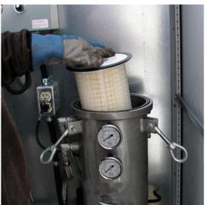
Step 9: Carefully tap the down the filter into the canister.
