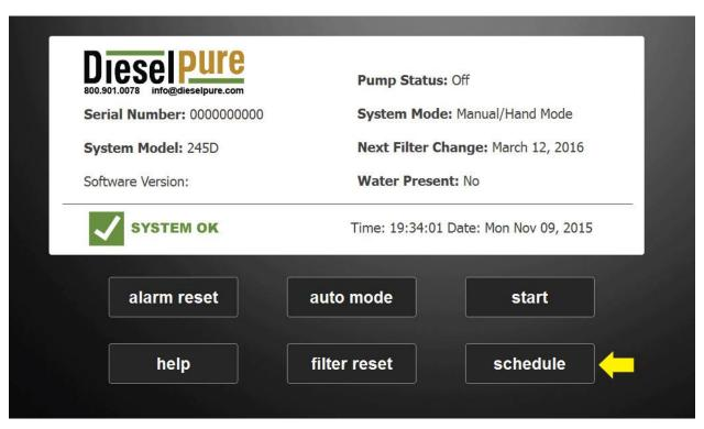
The schedule button is used to open the filter cycle scheduler
