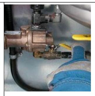
Step 3: Remove the "Water Drain Plug"
