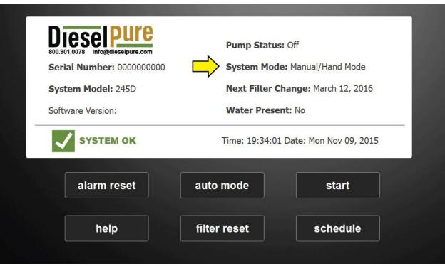
This area of the GUI indicates the current pump mode (Auto or Manual/Hand Mode)
