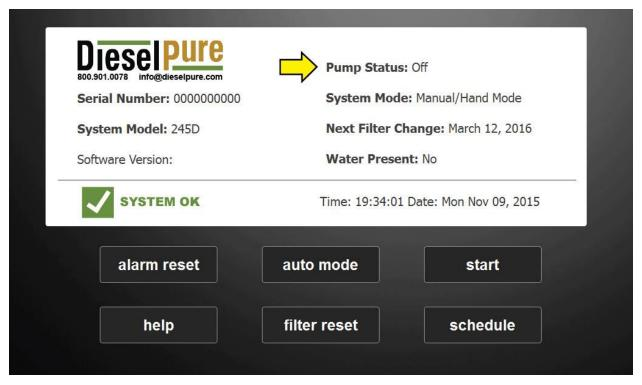
This area of the GUI indicates the current pump ON/OFF state.
