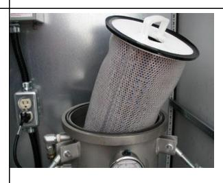
Lubricate the "O" ring with a bit of diesel
