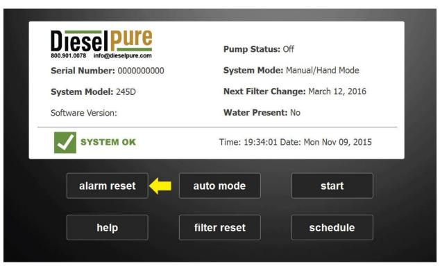
The alarm reset button used to reset the alarm status after a system fault has been corrected.
