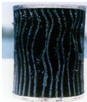
Diesel filter clogged with the "slime" resulting from microbial activity in the storage tank
