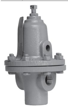
The Model BQ Back Pressure Regulating Valve is a self-operated spring-loaded back pressure regulating valve. Typically the Model BQ is installed at the far end of the oil supply line, down stream of the boiler fuel metering valves and passes unburned oil to the return line. Alternately, the Model BQ may be installed upstream of the boiler fuel metering valves. In both cases, the valve passes oil to the return line in order to maintain a constant supply pressure to the fuel metering valves.
