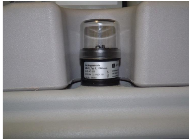
Photo F – To prevent spills, the Cube is constructed with double walls. If a leak within the inner wall were to occur, fluid would be visible in the sight glass. It is recommended that the sight glass be checked on a periodic basis.
