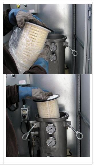
Step 9: Carefully tap the down the filter into the canister.
