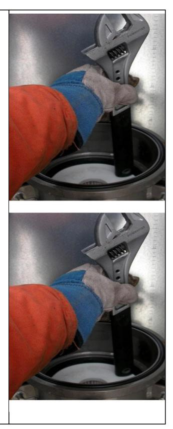
Step 9a: Check the water drain plug and ball valve to make sure they sealed and off.
