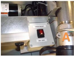
Photo A – Assure that the toggle switch is in the "ON" position.
