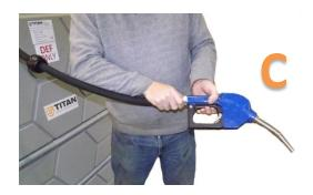
The dispense hose is connected to an integrated retractable hose reel. Only pull the hose from the reel using the installed ball stop mechanism.
