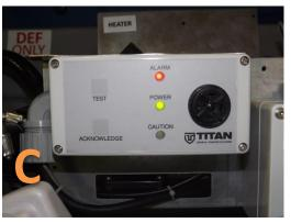
Photo C – Once the alarm has been silenced, the red alarm light will remain lit until the Cube is at less than 85% fill capacity.
