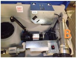
Photo C - Insert the nozzle in to the DEF tank of the vehicle to be filled. Depress the trigger on the nozzle to begin filling. When filling is complete, release the trigger and return the nozzle to its cradle on top of the Cube.
